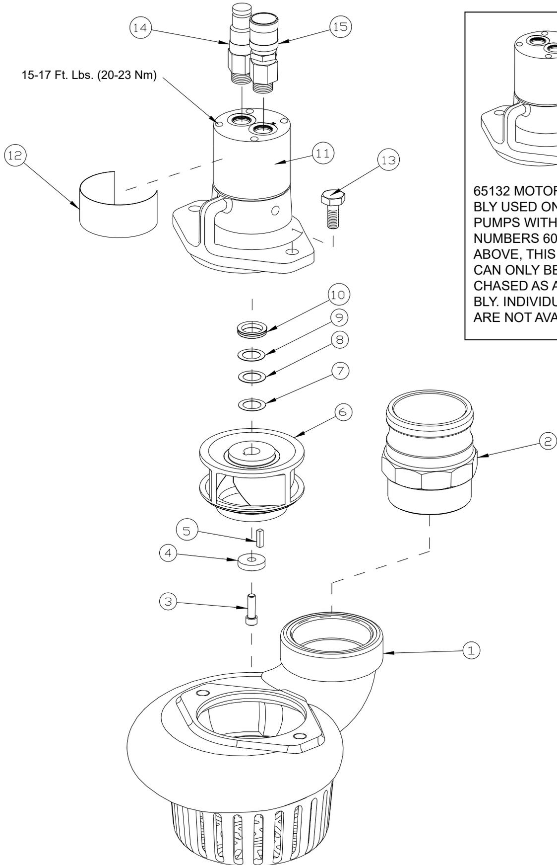
65132 MOTOR ASSEMBLY USED ON SUMP PUMPS WITH SERIAL NUMBERS 600 AND ABOVE, THIS MOTOR CAN ONLY BE PURCHASED AS AN ASSEMBLY. INDIVIDUAL PARTS ARE NOT AVAILABLE.
