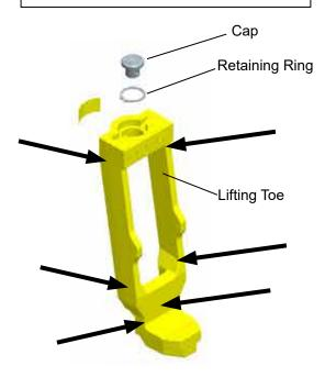
2. Once a month, remove the retaining ring and lifting toe. Thoroughly inspect the back, as well as the front and sides, for damage or cracks. Take special note of the areas indicated above.
