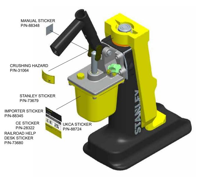
Note: The following information can be found on the bottom left side of the base. Model Number, Serial Number, 7250 PSI/500 Bar and year of manufacture are stamped in this location on each jack.
