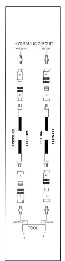
Figure 1. Typical Hose Connections
