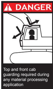
Top and front cab guarding required during any material processing application
