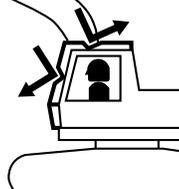
Top and front cab guarding required during any material processing application
